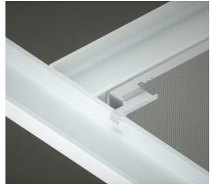
This is a hook-over bracket supplied fixed to the upstand of the panel. Access is obtained by pushing up the opposite end of the panel and sliding back. This reveals the flange which can then be lowered to a vertical position (lift & tilt).
