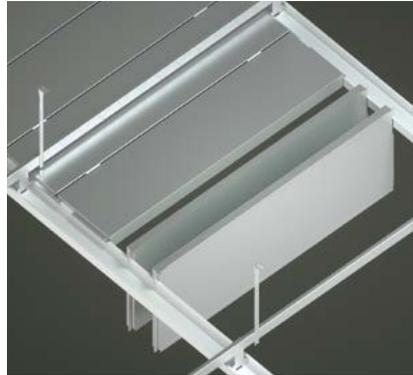
This integral feature allows tiles to be hung vertically from C-Profiles which provides unobstructed ceiling void access. Complete panel runs can be hung together during maintenance without causing damage to the tile.
