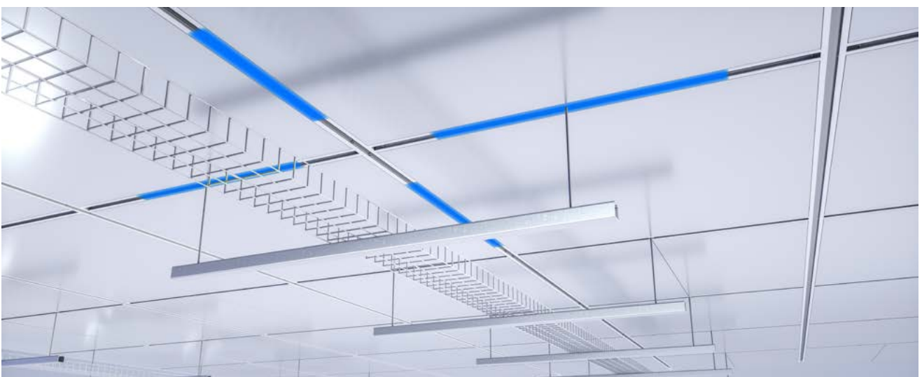
Load Case Zone 3 - 132lbs maximum anywhere outside of zone 2, where load must be in adjacent bays
