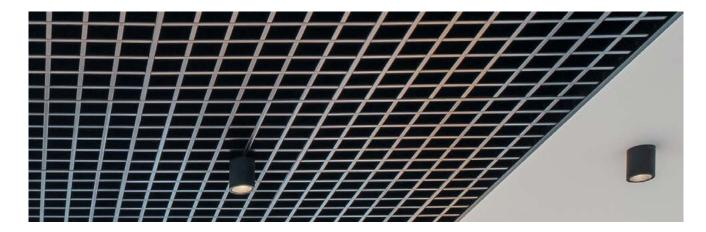
SAS800 Trucell is a decorative open cell ceiling, for airflow and smoke extraction applications. The metal ceiling system comprises a series of open cell modules designed to lay onto a suspension grid. The ceiling tiles can integrate within other metal ceiling systems and plasterboard ceilings.
