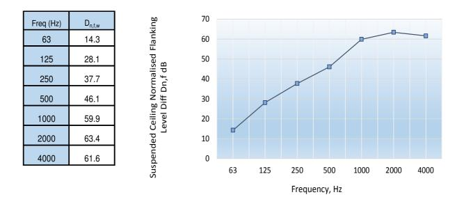
Single figure rating: D<sub>n,f,w</sub> (C;Ctr)= 49 (-2;-8)dB Rating according to BS EN ISO 717-1:1997
