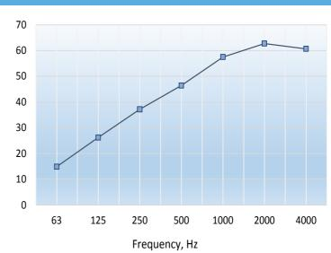
Single figure rating:  $D_{n,c,w}(C;Ctr) = 48$  (-2;-8) dB According to BS EN ISO 717-1: 1997
