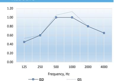
Single figure rating :  $\Omega\omega$  0.80 In accordance with BS EN ISO 11654: 1997
