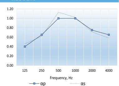
Single figure rating :  $\Omega\omega$  0.75(M) In accordance with BS EN ISO 11654: 1997
