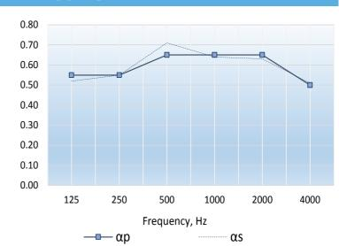
Single figure rating :  $\Omega\omega$  0.65 In accordance with BS EN ISO 11654: 1997
