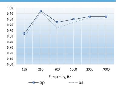
Single figure rating :  $\Omega\omega$  0.80(L) In accordance with BS EN ISO 11654: 1997
