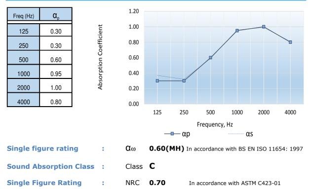
The measurement methodology and associated analysis results in absorption coefficients greater than unity. This is due to diffraction at the edge of the sample and is considered within the measurement standard by specifying the sample dimensions and perimeter detailing.
