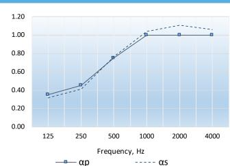
Single figure rating :  $\Omega_{\omega}$  0.75(L) In accordance with BS EN ISO 11654: 1997
