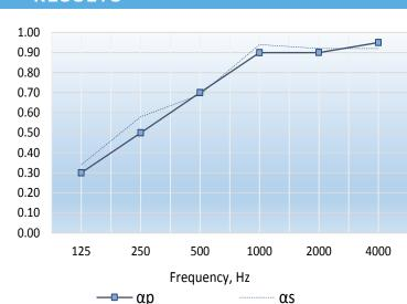
Single figure rating :  $\Omega_{\odot}$  0.75(H) In accordance with BS EN ISO 11654: 1997
