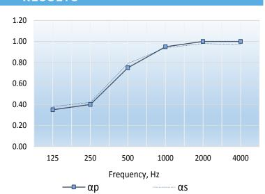
Single figure rating :  $\Omega_{\omega}$  0.70(MH) In accordance with BS EN ISO 11654: 1997
