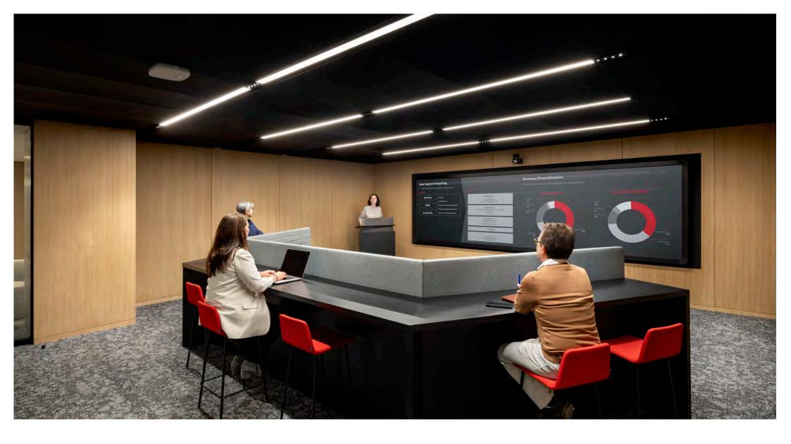
SAS International worked closely with TPG, who specified their linear raft SAS600 system in an expanded metal mesh finish. The layout of the rafts was carefully coordinated with the linear LED light fittings that sit in between each run of metal panels, each panel being fully accessible and polyester powder coat finished in RAL9005 black, providing a fresh and contemporary feeling to the JLL 'Tech Lab'.
