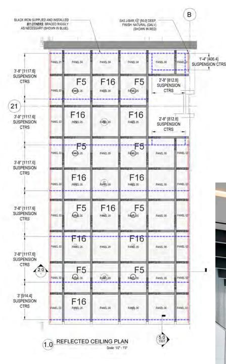
Alongside the workplace and amenity spaces, a design concept was developed for a geometric 'open grid' ceiling to the cafe. SAS International's design utilized the SAS500 baffle system, which was locked together using concealed bracketry, to form a series of boxes.
