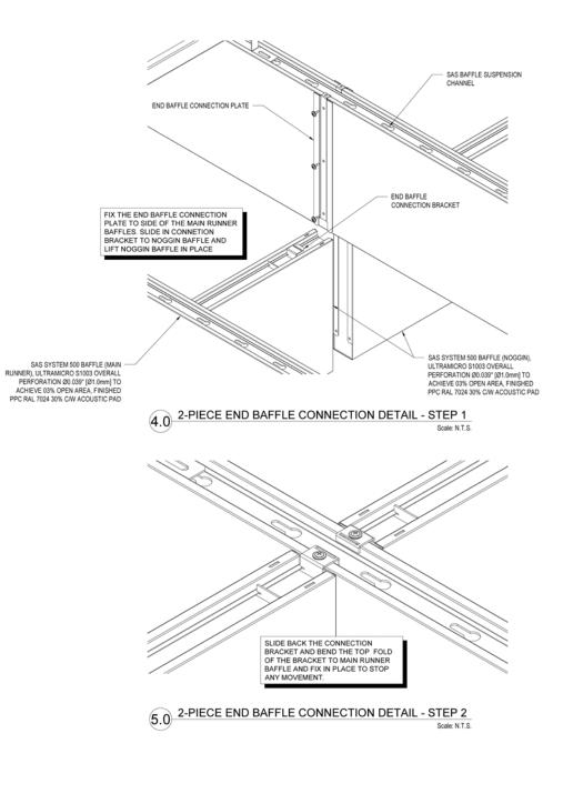
The parallel sides of each of the SAS500 baffles were perforated using SAS's S1003 ultra-micro perforation, as was the 'cap', and both were then supplied complete with SAS's high performance acoustic infill to deliver an NRC of 0.90.
