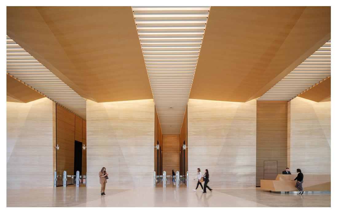
Designed by architects Goettsch Partners, the building's lobby features SAS's extruded aluminum SAS740 ceiling system finished in a soft champaign metallic matte above the elevator entrances. The design required close coordination with the lighting concept to effectively backlight the ceiling membrane for light reflectance and to add warmth to the space.
