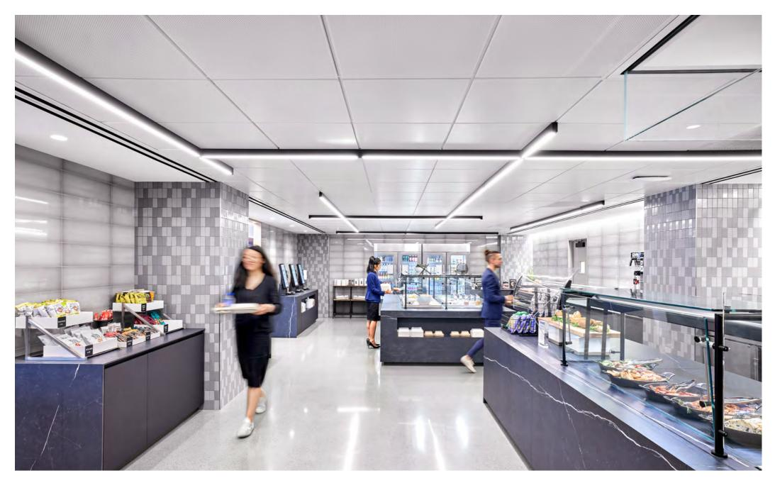
Finishing up the scope for SAS was the use of System 130 in the food servery area, installed on SAS's own 9/16" tee grid. The ceiling panels were perforated to D1505 to provide an NRC of 0.90 and were supplied complete with color matched aluminum perimeter trims.
