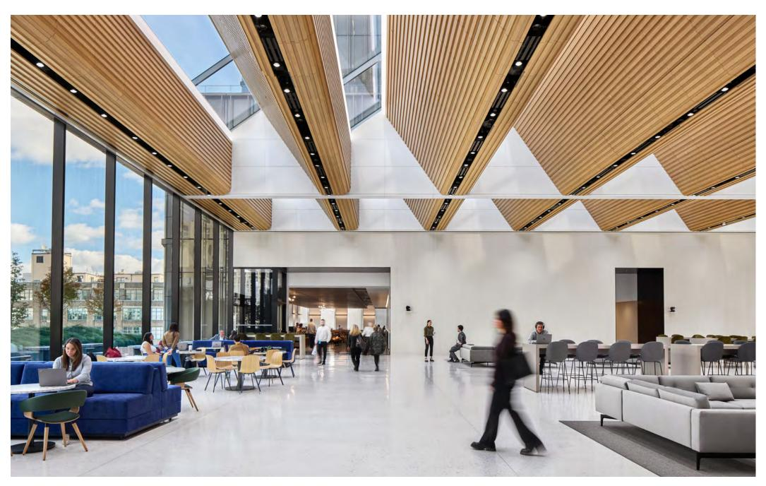
This scope was then complimented by plain white hook-on wall panels that run perpendicularly to the beam encasements. The final outcome was virtually identical to the Gensler rendering while providing the acoustic and access specifications required.
