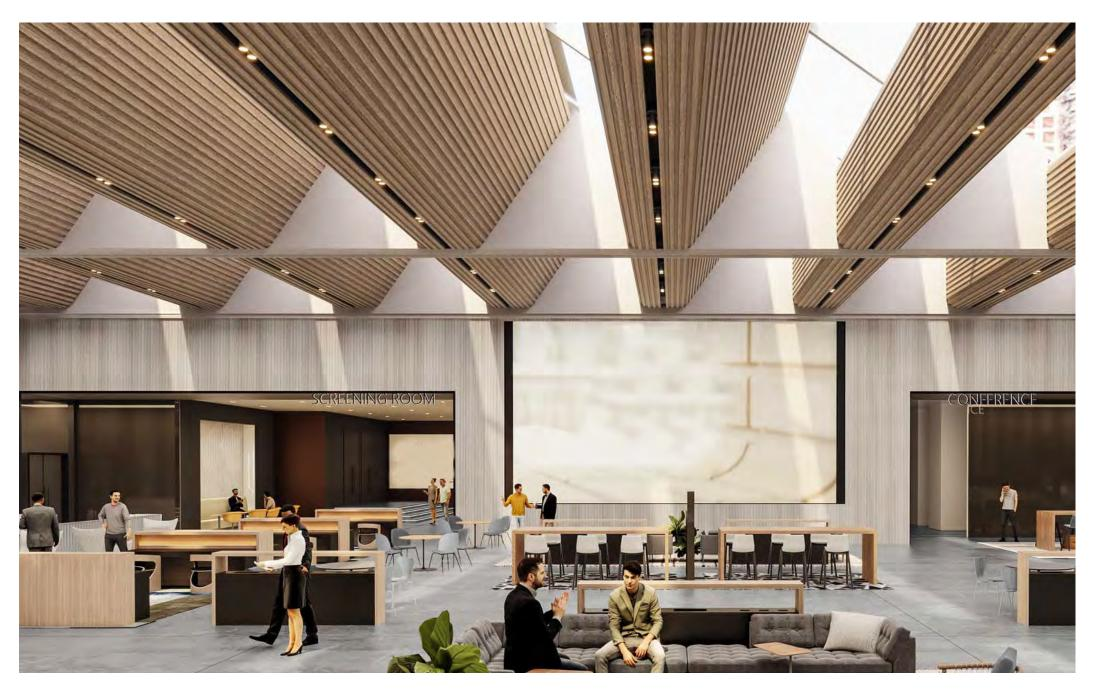
Within 'The Great Room' or Mixing Chamber, the brief and rendering (shown above) was to provide a corrugated, wood look, accessible and acoustic beam encasement. This contains the buildings structure as well as a host of mechanical and electrical services.
